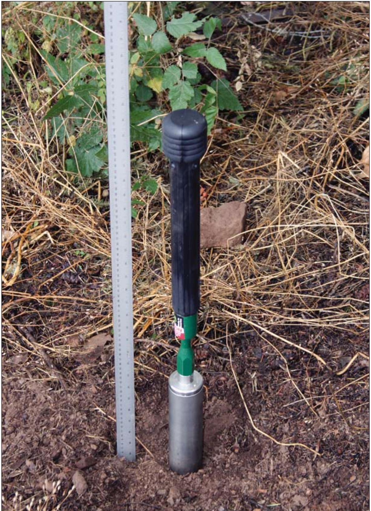
Figure 55—Forest soils are sampled with a soil coring device driven by an impact hammer.
