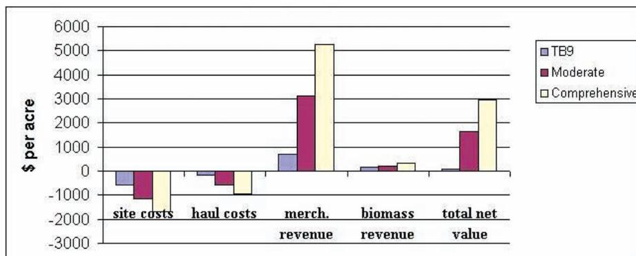
**Figure 2**—Costs, revenues and resulting net value for the three mechanical fuel treatment prescriptions applied where they result in positive returns. Site costs include merchantable (stump-to-truck) and any biomass removal (stump-to-truck and chipping) or preparation for pile burning. Haul costs include hauling merchantable material and biomass for biomass scenario. Merch revenue is the revenue for merchantable material.
