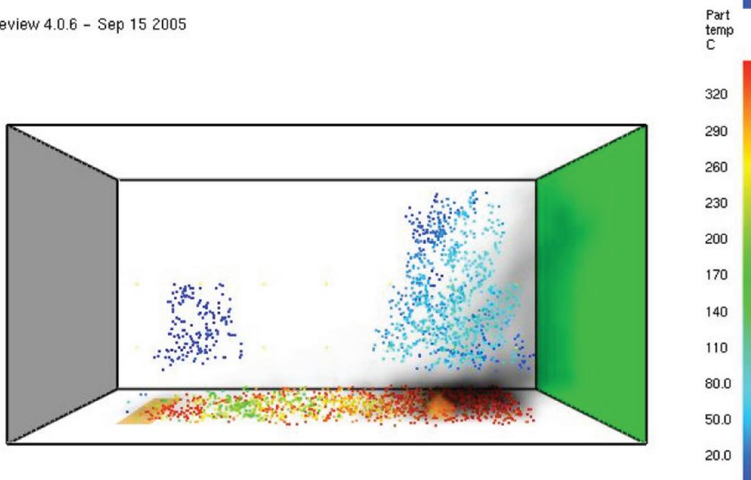
**Figure 10**—Demonstration of a numerical fire simulation with the Wildland Urban Interface Fire Dynamics Simulator (WFDS), and highly resolved fuels at t = 72 seconds. Surface fuels are burning in both simulations. Heat from the the middle dead tree in the untreated simulation (top), as well as from the surface fuels, has caused the tree at right to ignite, and it continues to burn intensely. In the “treated” simulation (bottom) the tree at right is scorched from below but does not ignite.
