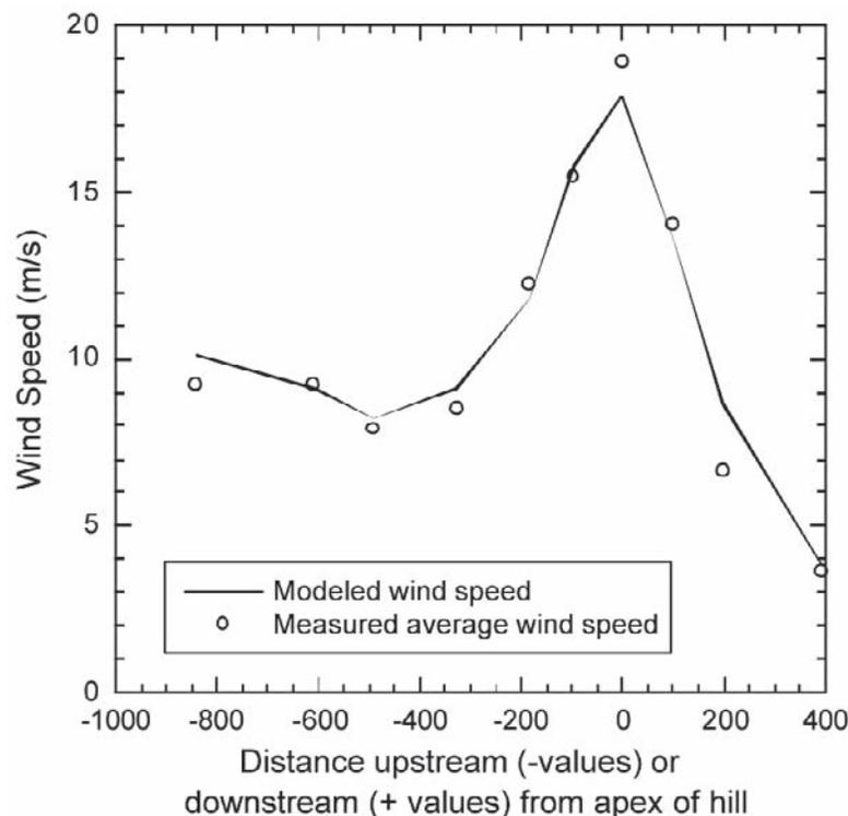
**Figure 2**—A comparison of measured and predicted wind speeds reported from the Askervein hill data set. Positive values represent distances downstream from apex and negative values represent upstream from apex.
