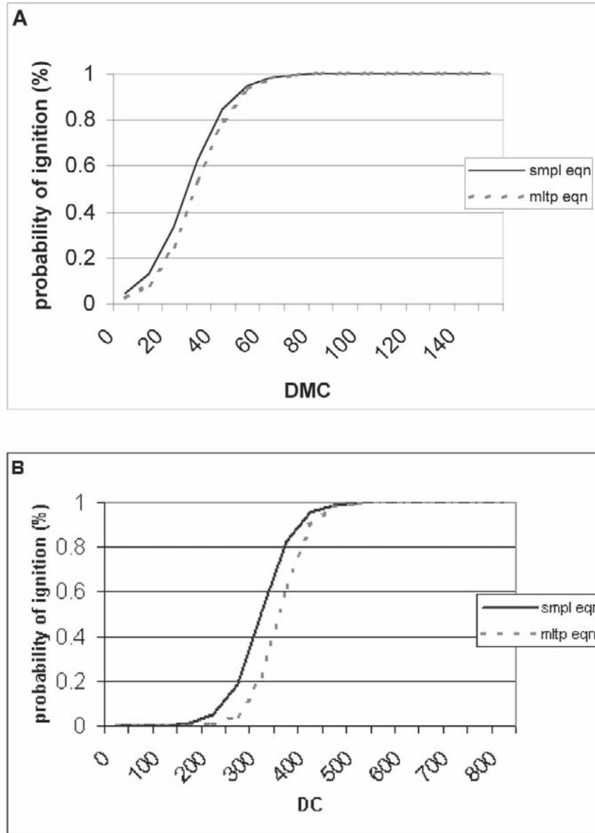
**Figure 1**—Results of the non-linear analysis fitted to a logistic model showing the probability of sustained ignition against the DMC (A) and DC (B) for simple (smpl) and multivariate (mltp) equations.
