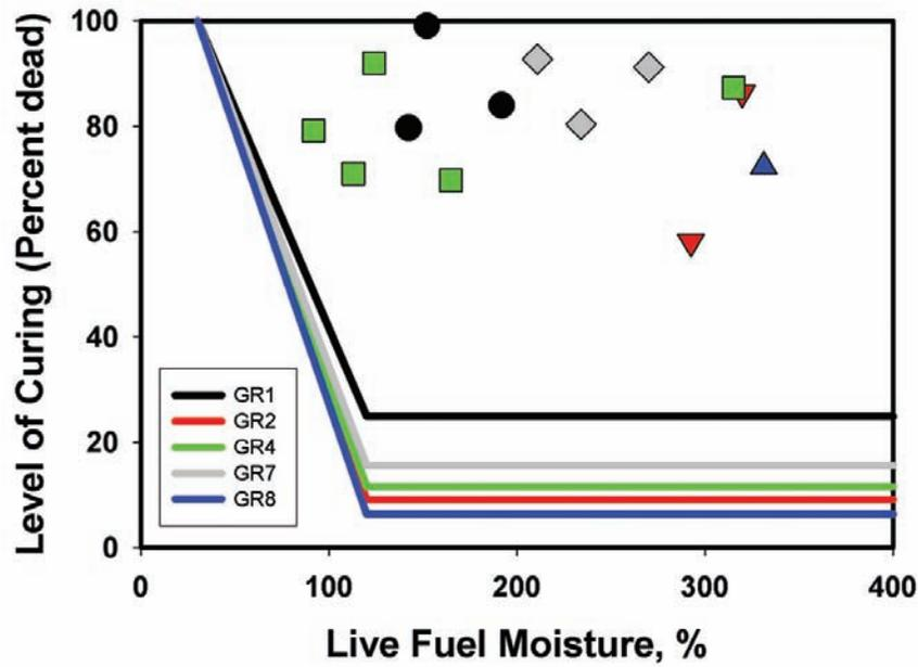
Figure 3—Australian and New Zealand live fuel moisture and curing data compared to the dynamic load transfer function. There is a different curve for each fuel model because of the dead fuel in the fuel models when there is zero load transferred from live to dead. The sample data points are from table 3.
