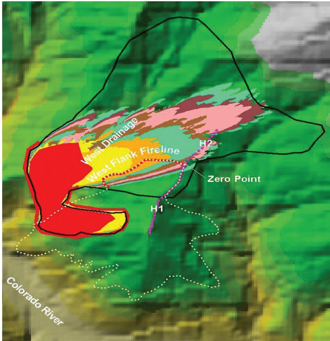
**Figure 4**—FARSITE simulation of the Storm King Mountain Fire assuming uniform wind speed and direction from the left to right (west winds). Black line represents actual fire perimeter at same point in time as last fire simulation. Fire growth simulations are shown as successive fire burned areas with color varying. Last perimeter is shown in light blue-green.
