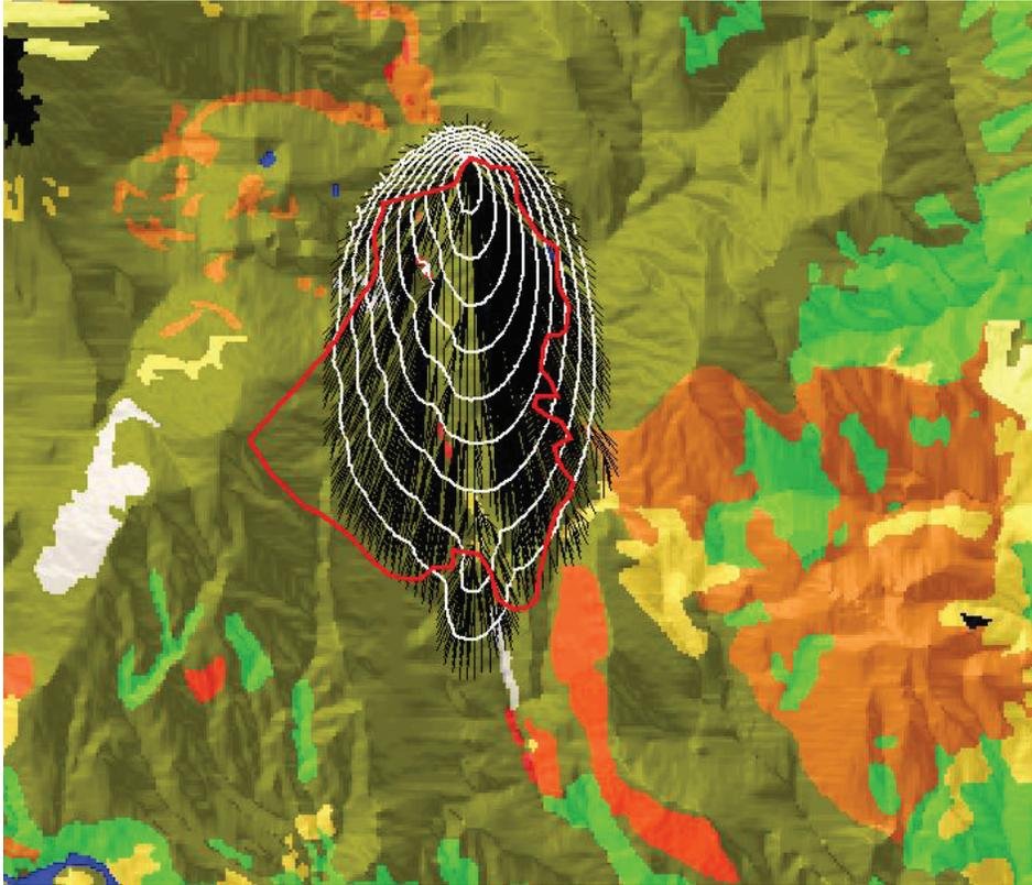
**Figure 2**—The Minimum Travel Time (MTT) model shows a slightly different shape for the New Zealand Craigeburn Fire. Although it uses the same fire behavior models as FARSITE, it propagates fire through regularly spaced nodes (Fermat's principle) rather than wave fronts (Huygens' principle) and uses constant rather than varied wind and weather inputs.
