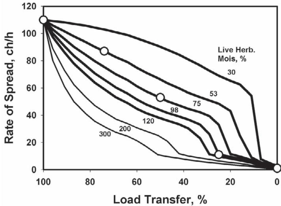
Figure 7—Rate of spread is calculated for several values of live herbaceous moisture for a range of load transfer percentage. Use of the load transfer function results in only the single indicated point on each curve. The curves correspond to the rows in table 5.
