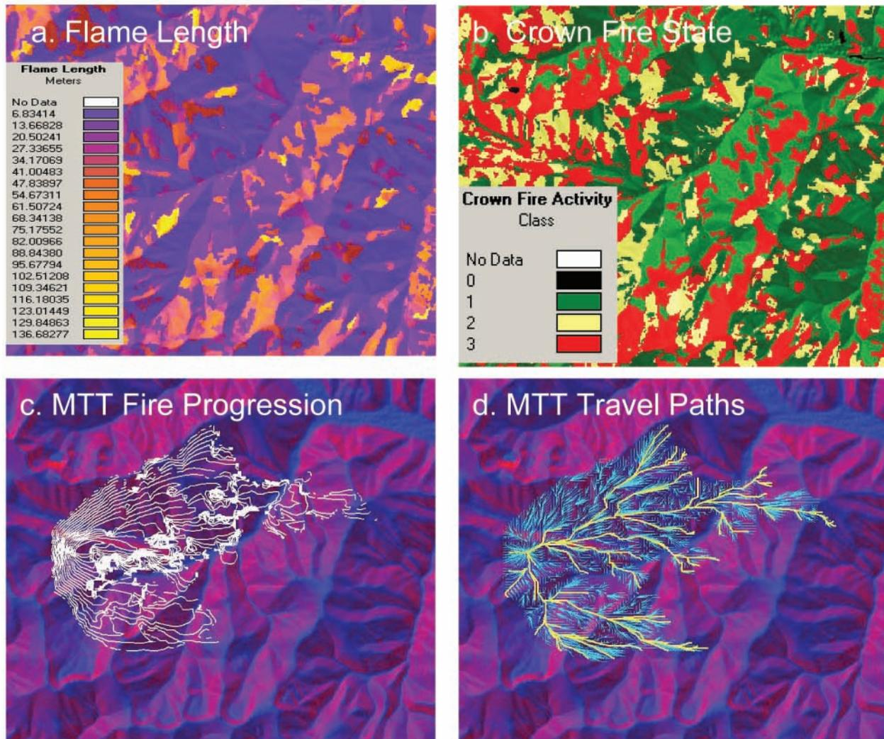
**Figure 2**—Example outputs from FlamMap for (a) fire spread rate, (b) crown fire activity (0=none, 1=surface fire, 2=torching trees or passive crown fire, and 3=active crown fire), (c) fire progression (white perimeters) simulated using the Minimum Travel Time (MTT) method, and (d) the fire travel paths produced by MTT (bold yellow lines distinguish major paths from all paths in light blue).
