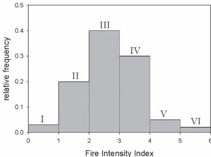
**Figure 3**—Relative frequency of Fire Intensity Index (the common logarithm of fireline intensity) given that a fire does occur at a given point. The sum of probabilities of observing individual FII classes is one. Relative frequency of FII is a function of the local fire environment at the time of the fire and the distribution of fire intensity at different parts of an assumed elliptical fire. FII class is indicated in Roman numerals.
