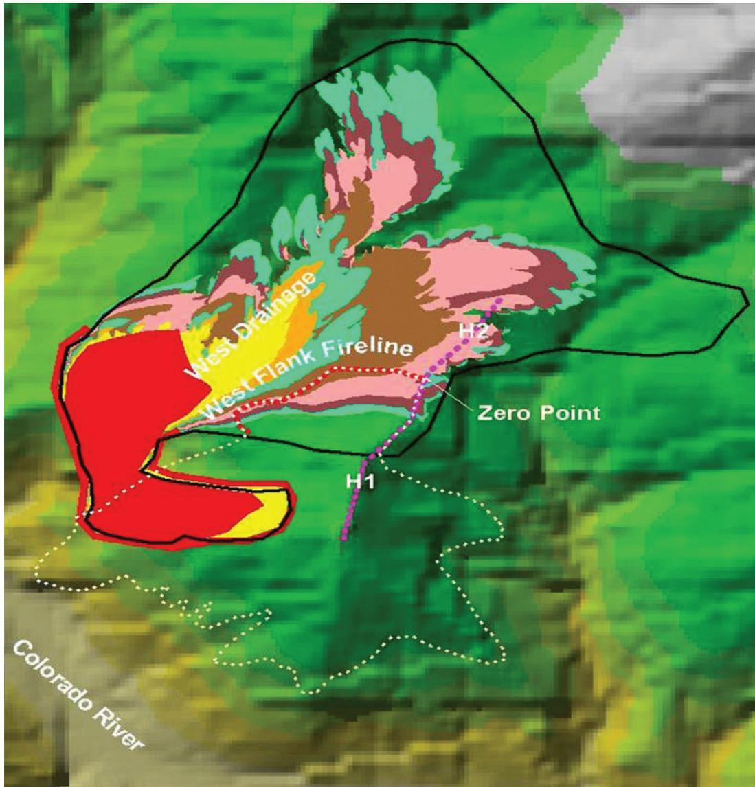
**Figure 5**—FARSITE simulation of the Storm King Mountain Fire using gridded wind data from CFD-based simulation. General wind flow input to CFD was aligned with the Colorado River gorge (west winds generally flowing diagonally from upper left to lower right). Black line represents actual fire perimeter at same point in time as last fire simulation. Fire growth simulations are shown as successive fire burned areas with color varying. Last perimeter is shown in light blue-green.
