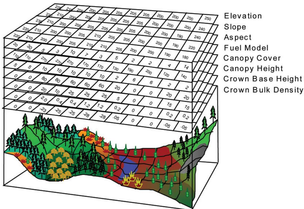
**Figure 1**—Input data themes required for running FlamMap are the same as those for FARSITE and are contained in a “Landscape” file constructed from ASCII Grid files that are of identical resolution, co-registered, and of equal extent.
