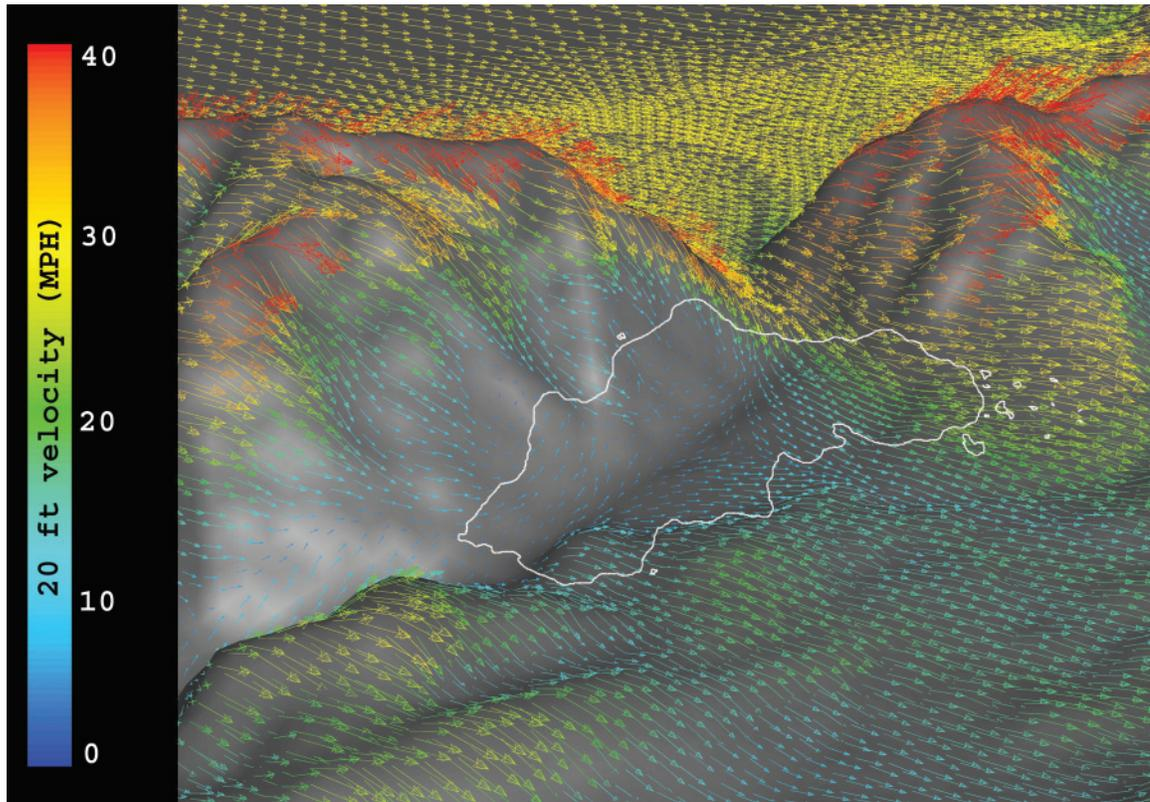
**Figure 1**—Example of a gridded wind simulation. The white line represents the fire perimeter. Wind speed and direction are indicated by the vectors, with length representative of relative speed and orientation representative of local wind direction. Vectors are also colored by wind speed.
