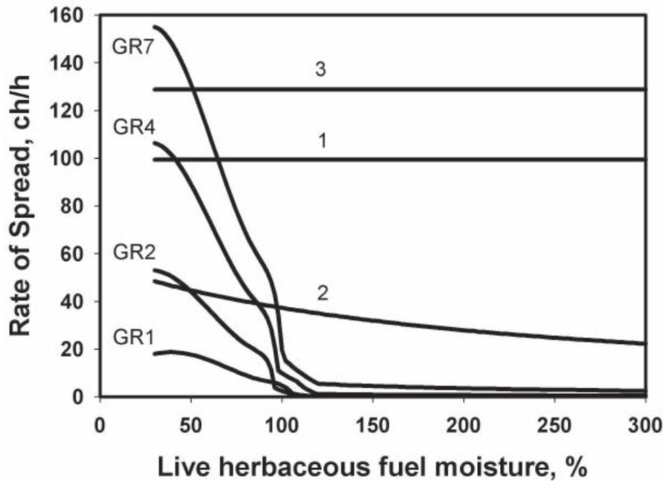
**Figure 2**—Comparison of calculated rate of spread for seven fuel models to illustrate sensitivity to live fuel moisture for static (1, 2, 3) and dynamic (GR1, GR2, GR4, GR7) fuel models. Dynamic fuel models include the use of the load transfer function.
