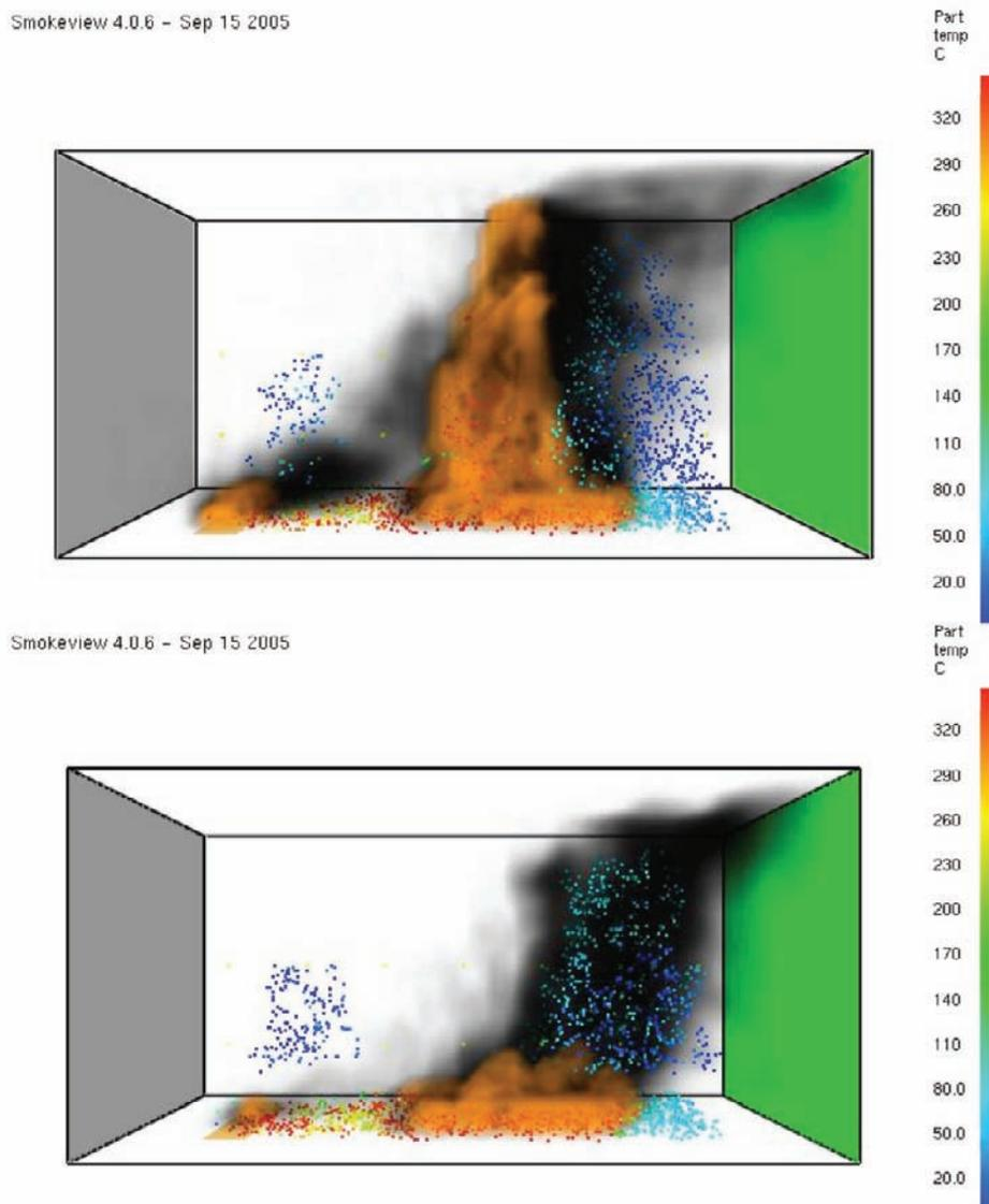
**Figure 8**—Demonstration of a numerical fire simulation with the Wildland Urban Interface Fire Dynamics Simulator (WFDS), and highly resolved fuels at  $t = 48$  seconds. Surface fuels are burning in both simulations but the middle dead tree in the untreated simulation (top) is burning intensely.
