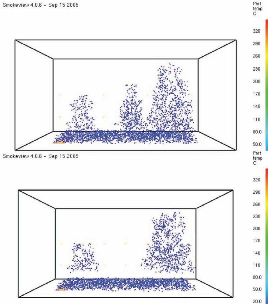
**Figure 7**—Comparison of two simulations with a numerical fire model, WFDS, and highly resolved at  $t = 0$ . Top figure shows “untreated” simulation with three small trees and a surface fuel bed in a wind tunnel. The outer trees are live, with high moistures and the middle tree is dead with low moisture, representing a recently bug-killed tree. Bottom figure shows the “treated” simulation in which the middle dead tree has been removed and lower branches have been pruned to 0.75 m.
