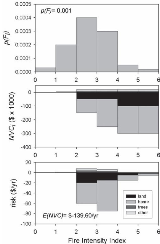
**Figure 4**—A “Riskogram”—a graphical display of the elements of a quantitative fire risk analysis. Chart (a) displays the frequency distribution of the Fire Intensity Index (FII) at a point. The sum of probabilities in individual FII classes is the annual probability of burning. Chart (b) displays the predicted net change of different values to fire of the various FII classes. Chart (c) displays the resulting wildland fire risk. The sum of  $E(NVC)$  over all FII classes is wildland fire risk.
