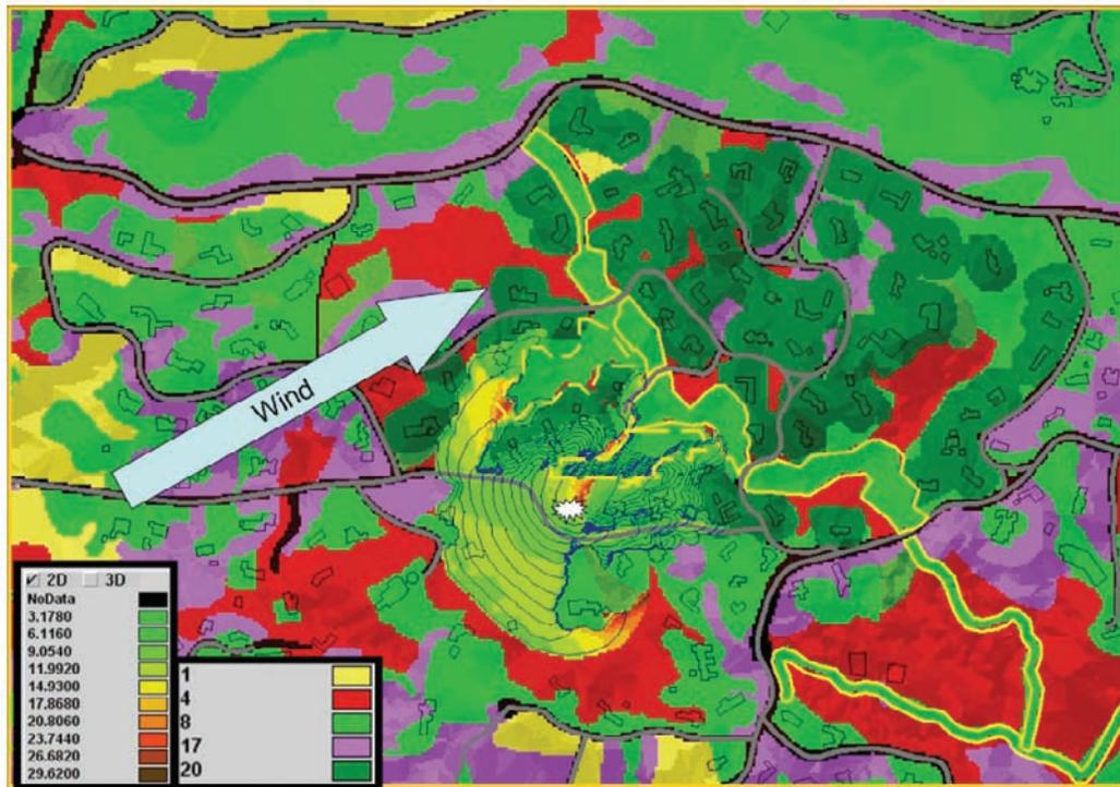
**Figure 5**—Post-treatment FARSITE simulations from a single ignition point under 97<sup>th</sup> percentile weather and wind conditions (August).
