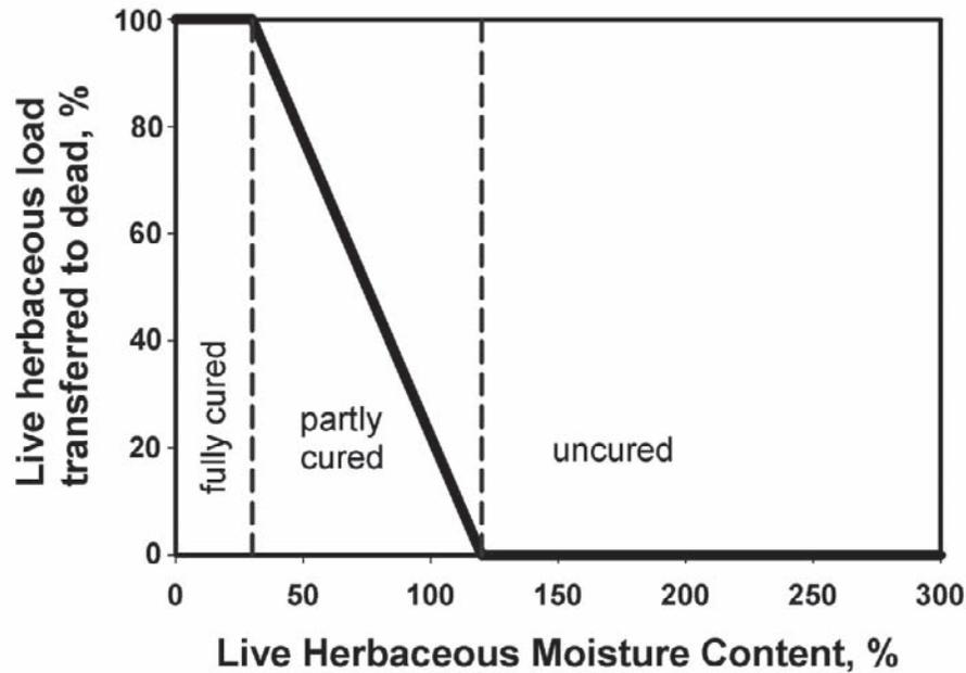
**Figure 1**—Percent of the live herbaceous fuel load that is transferred to the dead category (Burgan 1979). There is dead fuel in the fuel model when the percent is zero, for the section of the graph labeled “uncured.”
