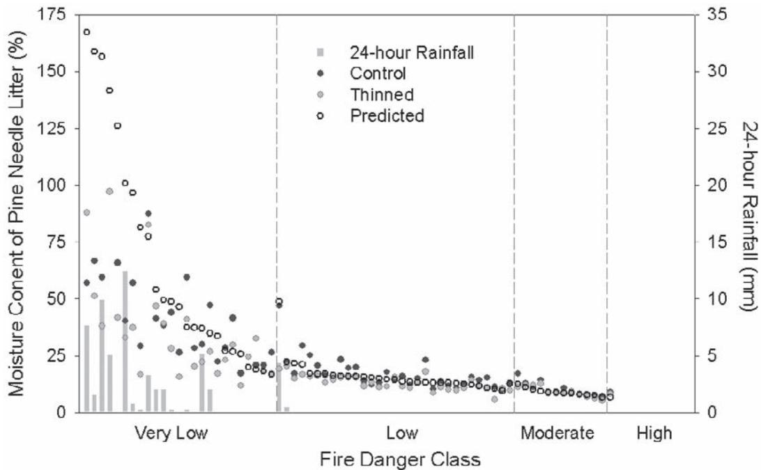
**Figure 11**—Predicted and actual mean moisture content (percent) of lodgepole pine needle litter in the thinned and unthinned stands, plotted from wettest to driest predicted value within different Fire Danger Classes, with corresponding 24-hour rainfall (mm) shown as bars.
