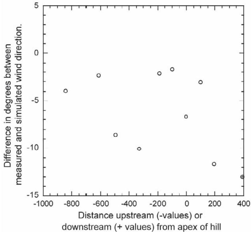
**Figure 3**—A comparison of the variation from the overall 210 degree flow direction for the measured and predicted winds from apex of Askervien hill. Positive values represent distances downstream from apex and negative values represent upstream from apex.
