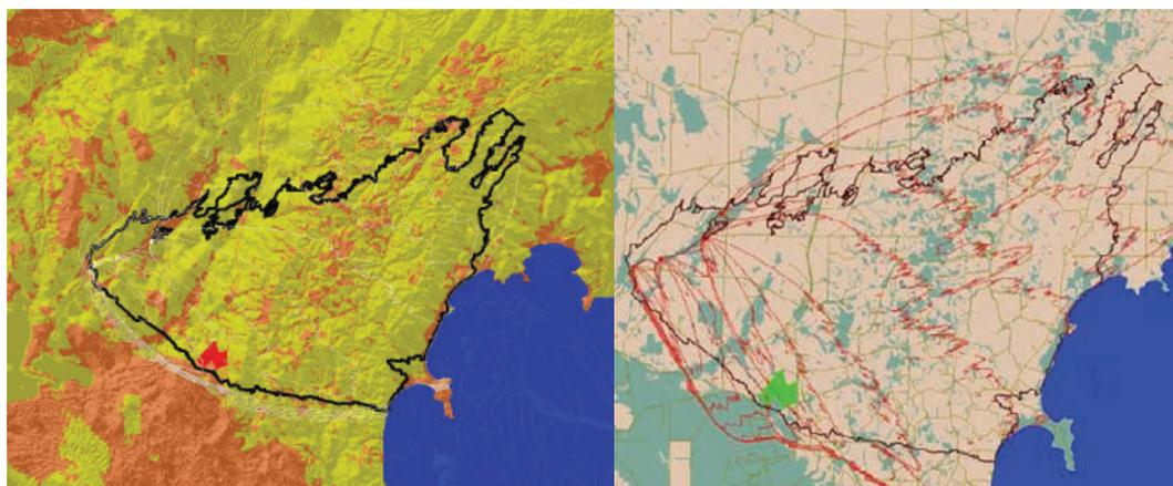
**Figure 3**—FARSITE (left) and Prometheus (right) modeled Australia's Wangary Fire. Although there are differences in the fire spread model, how suppression was modeled in each simulator, and the starting times of the spot fires, the resulting perimeters still coincide reasonably well with the final fire edge (black).
