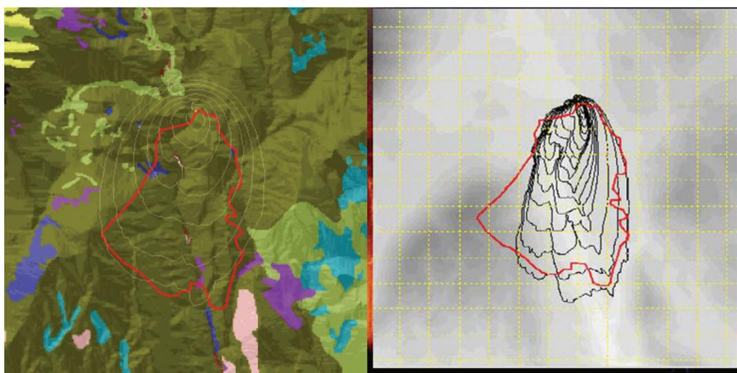
**Figure 1**—For the New Zealand Craieburn Fire, FARSITE (left) simulated fire perimeters (white) against the final fire perimeter (black); Prometheus (right) simulated perimeters (black) against the actual fire (red). Both simulations are reasonable, especially if the effect of suppression is considered.
