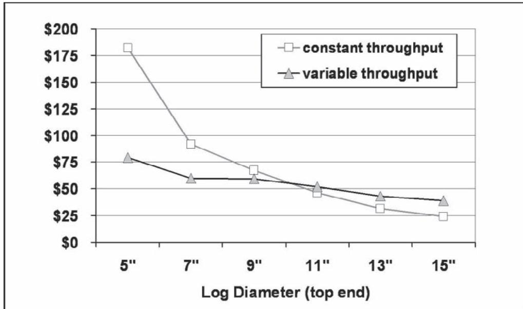
**Figure 5**—Non-wood lumber manufacturing costs (\$/thousand board feet) with constant log throughput and variable-speed log throughput assumptions.
