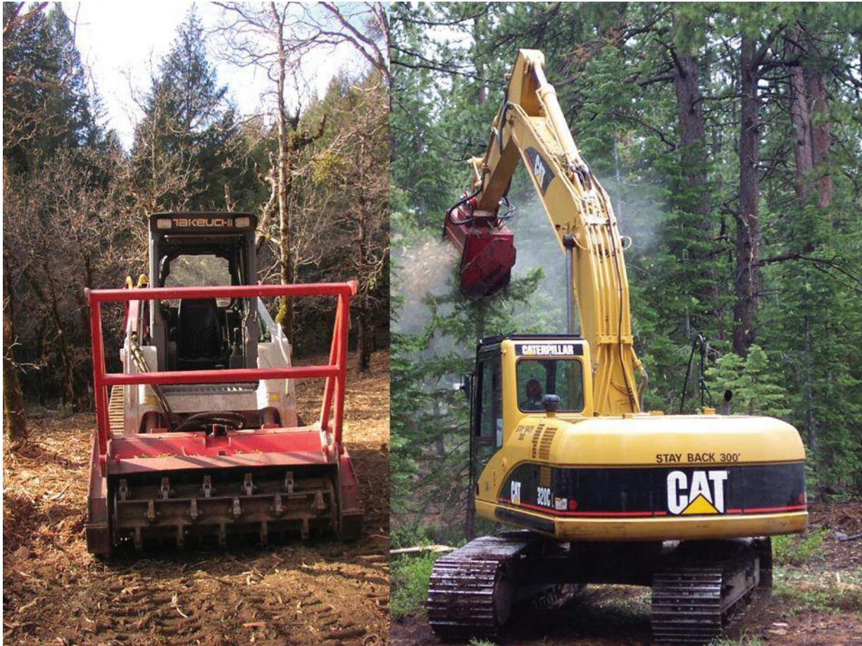
**Figure 1**—General masticator types: front-end mounted, Takeuchi®, TL150 w/ FECON Bull hog® shredder head (left) and a boom-mounted FECON Bull hog® shredder head mounted on an excavator (right). (left-Photo courtesy of Nancy Curran, USDA Forest Service).
