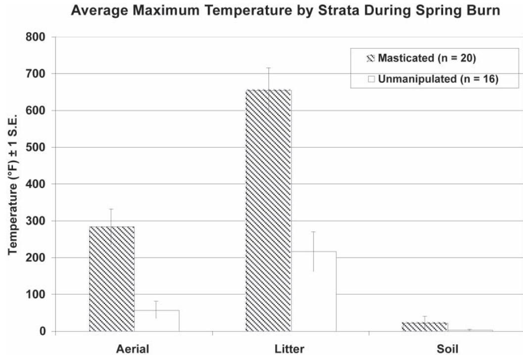
**Figure 2**—Average temperatures recorded by pyrometers during the burn treatment in masticated and unmanipulated plots. Aerial pyrometers were located 0.5 m/1.64 ft above the ground surface, litter pyrometers were located on the surface of the litter, and soil pyrometers were located between the duff and soil layers.
