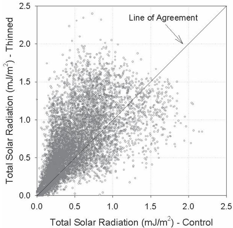
**Figure 7**—Total hourly solar radiation (mJ/m<sup>2</sup>) at 1.3 m height in the thinned stand, measured between 12:00 MST and 16:00 MST, vs. corresponding total hourly solar radiation in the control stand (n=8503 hours).
