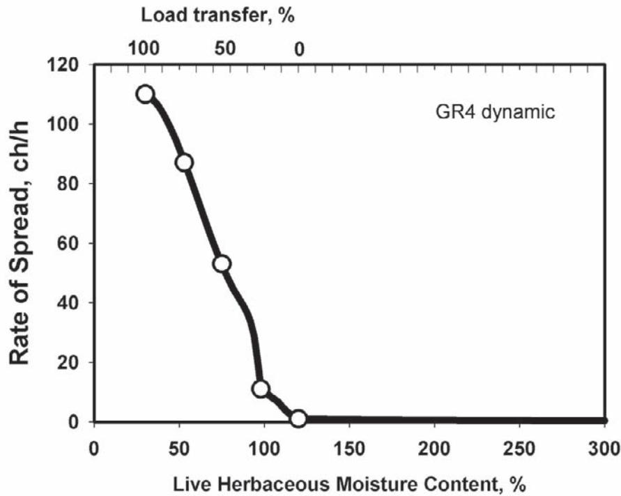
**Figure 5**—Calculated rate of spread for dynamic fuel model GR4, which incorporates the fuel load transfer function. Load is transferred from the live to the dead class as a function of live fuel moisture. The data points on the curve are given in table 4.
