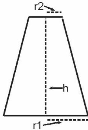
**Figure 3**—Planar view of a frustum of a cone, defined by length  $h$ , large radius  $R$ , and small radius  $r$ . The frustum of a cone is the basic building block for branches within the FUEL3-D spatial fuel model.
