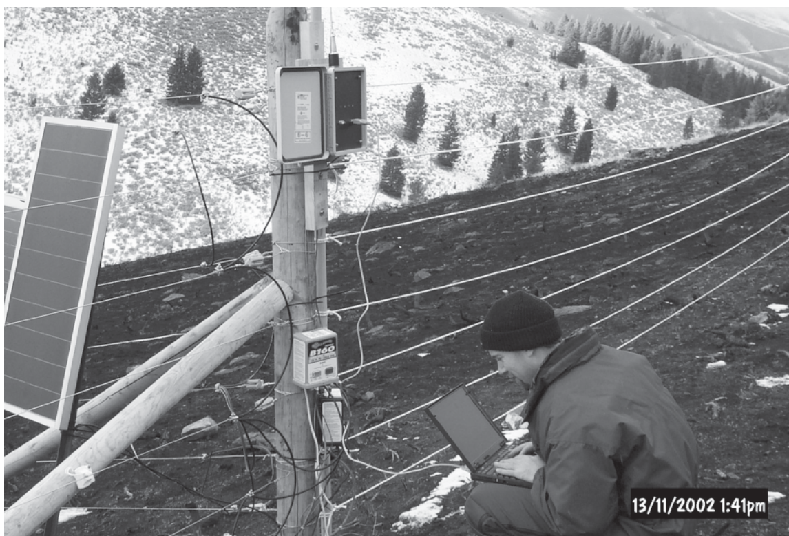
Figure 4 —MTDC evaluated nonelectric polymesh fence, polyrope electric fence, and high-tensile electric fence to exclude moose and elk from restoration areas.
