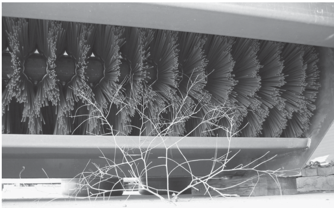
Figure 5 —Stiff bristles with convoluted wafers worked better than factory brushes to collect small forbs seeds on this Woodland Flail Vac brush harvester.
