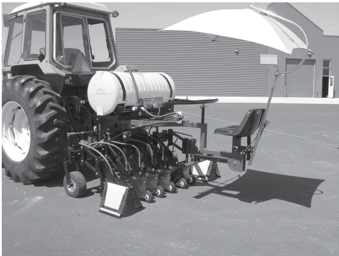
Figure 2 —An improved shielded herbicide sprayer, developed by MTDC, was evaluated in Virginia.
