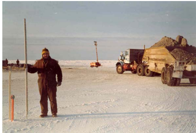
Deflection measurements with level and rod
