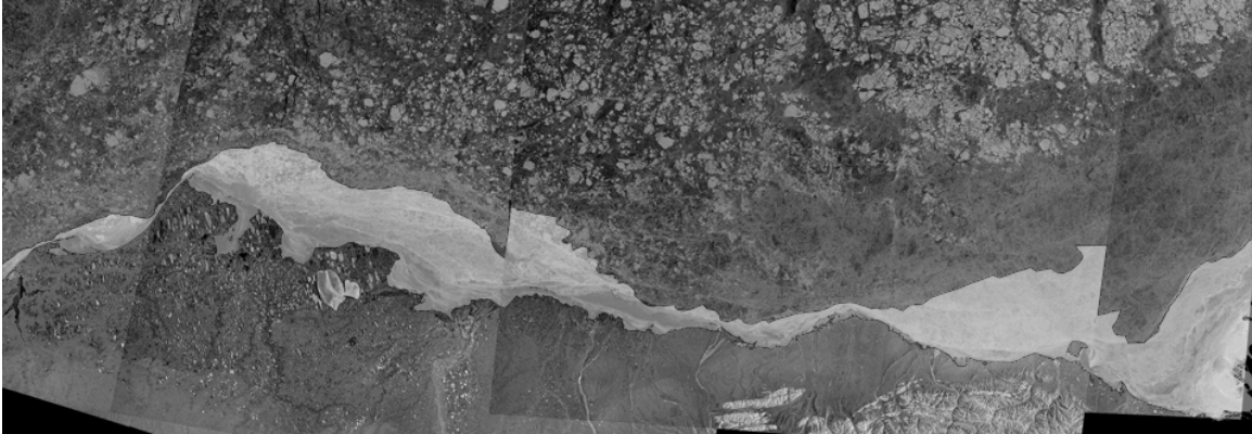
Figure 3.3.8: The landfast ice area for the period February 16 – March 8, 2000, overlain semi-transparently on the first of the 3 mosaics of period. This shows how mosaic boundaries, which effectively represent temporal boundaries in the image, lead to artifacts along the SLIE.
