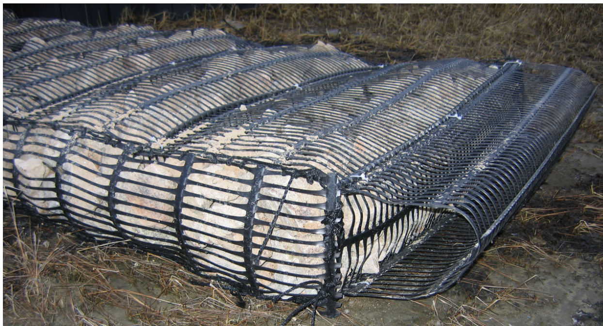
Figure 1. Portion of marine mattress showing geogrid container (photograph by Kevin Knuuti, Coastal and Hydraulics Laboratory (CHL))
