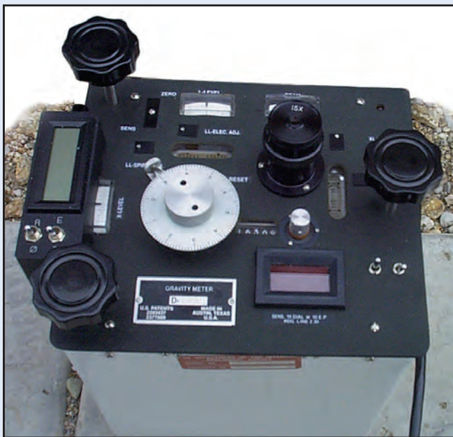
Gravity meter setup at a microgravity station. Photograph provided by Mark T. Anderson, U.S. Geological Survey.
