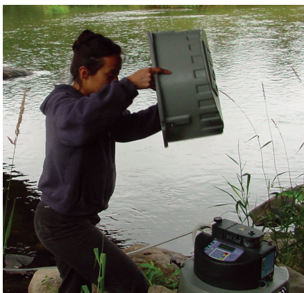
Cara O'Donnell, Water Quality Specialist for the Houlton Band of Maliseet Indians, retrieves river-water samples from an automatic sampler on the Meduxnekeag River, Maine. Photograph by Rhonda Jewell.
