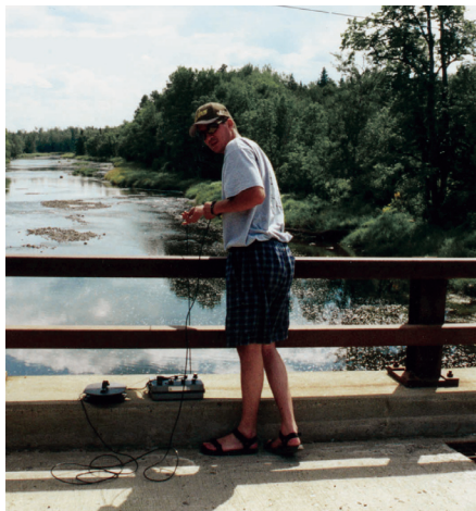
Dave Joseph, of the Houlton Band of Maliseet Indians, makes a dissolved oxygen measurement on the Meduxnekeag River, Maine. Photograph by Cara O'Donnell.
