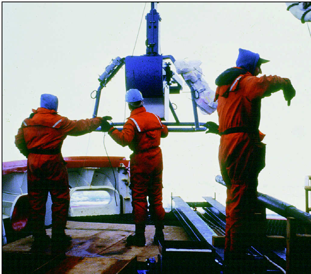
Preparing to send a giant box corer to the bottom of the Arctic Ocean. These cores provide relatively undisturbed sediment samples of the upper 50 cm of ocean bottom. Photo by Lisa Clough.
