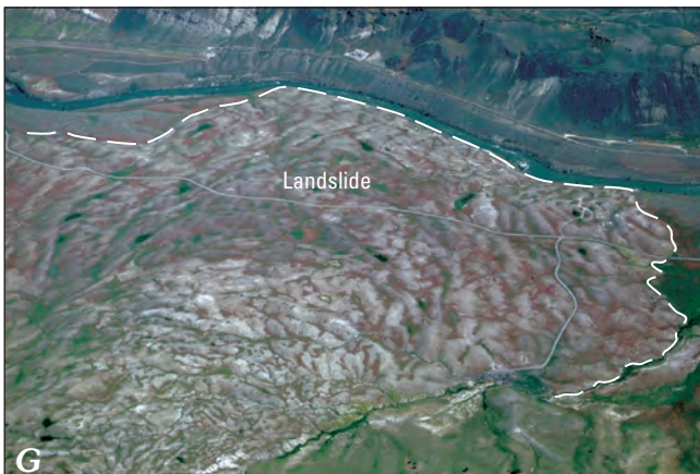
G, Landslide west of Gardiner, Mont., in incompetent, muddy sediments beneath slopes oversteepened by glacial erosion.
