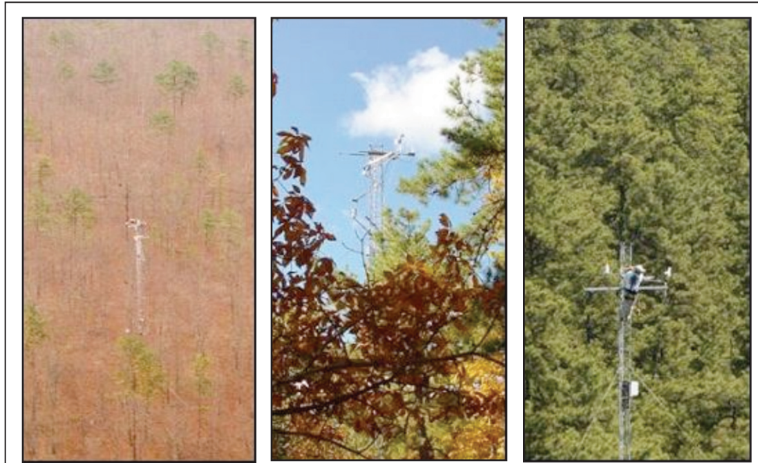
New Jersey towers located in (from left) oak/pine (leaf off), pine/oak, and pitch pine/scrub oak sites with instrumentation to measure: fire weather, fluxes of turbulence, energy, water vapor, and carbon dioxide. Photos: U.S. Forest Service.
