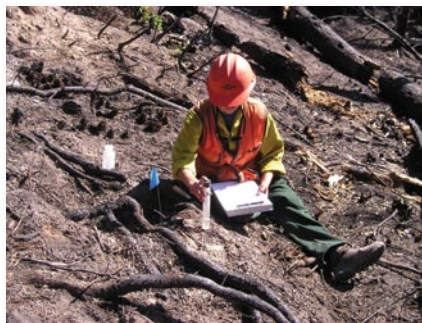
Figure 5. Sarah Lewis uses a mini-disk Infiltrometer (Decagon Devices, Pullman, WA) to measure a relative water infiltration rate to assess the degree of post-fire soil water repellency after the Robert Fire, Flathead National Forest MT. Photo by: Andrew Hudak (USDA FS), 2003
