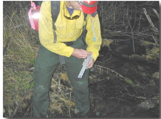
Figure 2. Damien Cremins, fire technician, measuring and counting pebble size in a tributary of Fish Creek in the Lolo National Forest, MT. Photo by: Matt Burbank (USDA FS), 2003.
