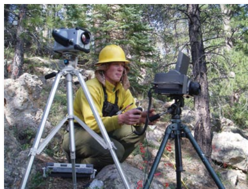
Figure 7. Patrick Freeborn installs and operates mid- and short-wave thermal infrared cameras to monitor radiant heat flux and temperatures within the Rapid Response Research plots on the Dragon Complex Wildland Fire Use Incident, North Rim of the Grand Canyon, AZ. Photo by: Colin Hardy (USDA FS), 2005.
