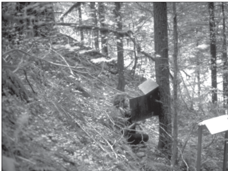
Figure 55—Bill Emmingham took this photo of his graduate advisee, Gabriel Tucker, working at a field site on Watershed 10 in May 1975 during the International Biological Programme. In the photo, Tucker is changing the chart on the circular thermograph recorder used to measure soil and air temperature. Two decades later, Tucker returned to work with the Andrews group.
